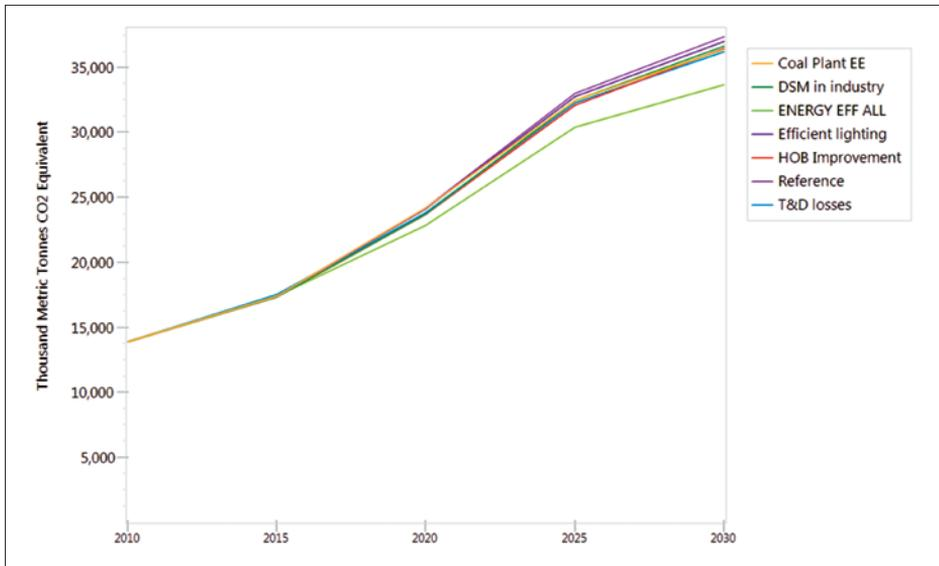
Figure 7.26 Scenario for efficiency improvements in power plants HOBs and utilities
