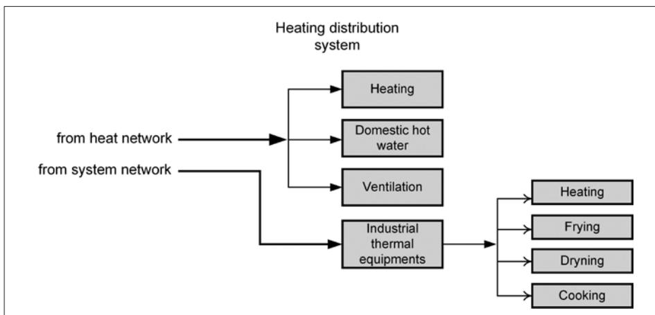
Figure 8.8 Structure of heat distribution system
