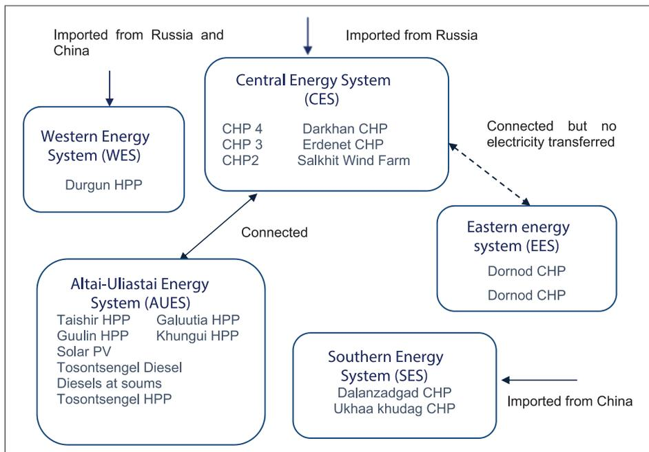
Figure 6.1 Electricity supply system of Mongolia
